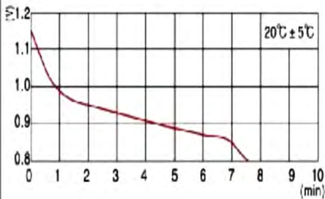
51A discharge curves of high discharge rate Ni-cd battery
